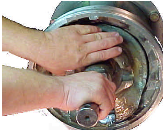
Step 11. Remove the #2937 spacer collar.
