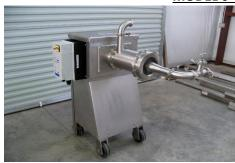
This machine regrinds the product from the bone collector through a 1/16" hole plate, which has another bone collector on it (regulated by a manual valve). It is controlled by a Lenze NEMA-4X washdown duty inverter so it can be slowed down or sped up to control the amount of product that flows through the bone collector on the final grinder. it is powered by a 7.5 hp Leeson motor and Cone Drive gearbox.
