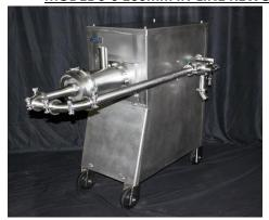
On this option, the Regulator 2" Rotary Bone Valve is built into the side of the Model 6-6 160mm In-Line Rework grinder. It is also controlled by a Lenze NEMA-4X washdown duty inverter and offers the best combination of bone collection control and rework capabilities. It is powered by a 7.5 hp Leeson motor and two Cone Drive gearboxes.
