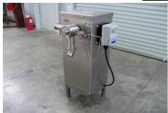
This is basically a slow turning vane pump. It has a Lenze NEMA-4X washdown duty inverter on it so you can control how much product is expelled through the Bone Collection Assembly. It does not rework the product from the bone collector, but it is an excellent way to control it. It is powered by a 1 hp Leeson motor and a Cone Drive gearbox.
