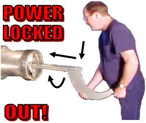
If the feedscrew does not slide up on the spline, it may be necessary to push down and in, while turning the feedscrew slightly to engage the drive spline. B drives engage easier than the older A drives. Never reach into the hopper to engage the drive spline. The feedscrew will jump in another inch when it is seated on the spline. Check the head space!
