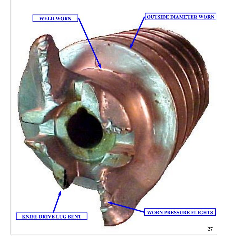
Examine the flights in the head section. Notice how the corners are rounded. The flighting should be replaced when it is worn down to 3/8" thick. Also notice the crack at the root of the shaft. There is so much wear of the weld that holds the flighting to the shaft that it is prone to cracking. A feedscrew with this amount of wear requires all new flighting. When we replace the flighting we machine the old flighting off, right down to the shaft. The flighting is replaced with new 1045 bar.
