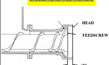
The head space should be checked on a weekly basis. The head space is 3/4" on all DGI grinder units. This should be done with the excluder seal removed. Spacers should be added if the measurement is more than 3/4". Spacers should be removed if less than 3/4".
