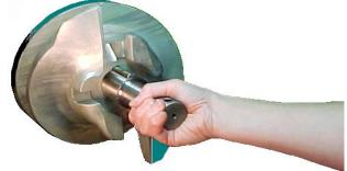
Insert the pin in the pin hole of the feedscrew. As you push the pin in, line up the key with the keyway. The pin bottoms out in the hole in the feedscrew. The pin should slip in by hand! If it does not check the pin hole for nicks and foreign material.
