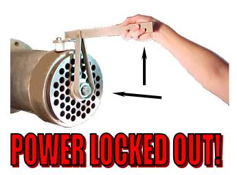
Slide the orifice plate with the plate bushing installed over the end of the grinder pin. Lift the end of the plate lifter handle and push the plate into the grinder unit.
