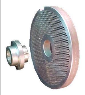
**Step 12.** INSTALL PLATE AND BUSHING INTO GRINDER UNIT.
