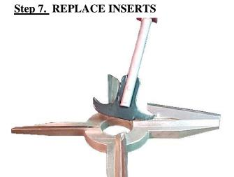
Inserting the pointed end of our insert remover into the slot of the knifeholder provides a quick and easy way to remove the knife inserts. Removing them in this manner minimizes damage to the insert locating pins found in the bottom of the insert slots in the knifeholder. We recommend starting with fresh inserts at every plate change! This includes when turning the plate around.
