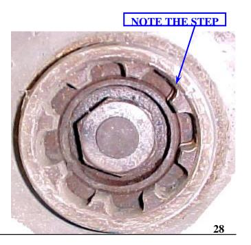
Note the sharp corners and square edges on a new feedscrew.
