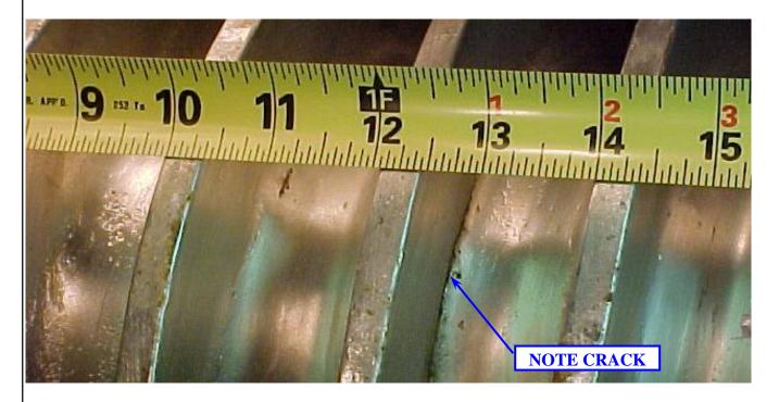
Examine the cupping. The cupping should have a sharp edge, so that it can aggressively capture the product being ground. When the cupping becomes dull the product is prone to rolling in the hopper.
