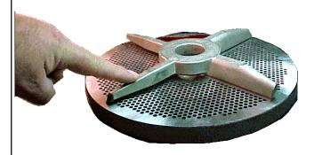
The combination of the insert slot angle and the angle that the inserts are ground provide that only the leading edge of the knife insert contacts the plate. This slight amount of clearance allows the insert to seat within a few revolutions of the grinder being turned on. The amount of material removed from the leading edge of the insert is not measurable, but it is advised that the first product that comes out of any meat grinder on start up is discarded.
