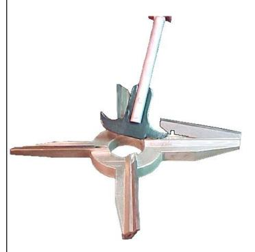
With the inserts out, inspect the slots. Every knifholder has a pin that lines up with a notch in the knife insert. If the inserts are removed incorrectly these pins can be broken. Send your knifeholder with broken pins to Dixie Grinders Inc. for repair.
