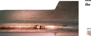
Examine the knife inserts. The edge of the insert should be free of burrs, Be carefull, the inserts are sharp!
