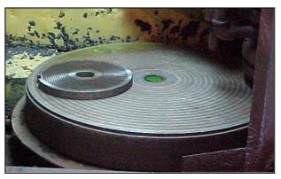
Rather, place the plate over the center of the surface grinder table, like this!
