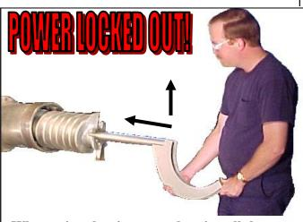
When using the ring wrench to install the feedscrew, lift the feedscrew slightly while pushing it in.
