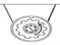
ROTATION: When the grinder unit has been disassembled, and then wired according to all applicable codes and regulations, rotation can be checked. Do not turn the unit on until you are positive that no one is in harms way! The grinder feedscrew should turn counterclockwise! After the rotation has been checked LOCK OUT THE POWER!
