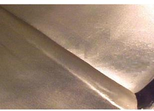
Detail of rebuilt spin ridge, note the sharp corner.
