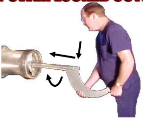
If the feedscrew does not slide up on the spline, it may be necessary to push down, in, while turning the feedscrew slightly to engage the drive spline. B drives engage much easier than the older A drives. The feedscrew will jump in another inch when it is seated on the spline.
