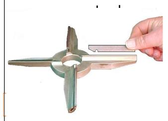
When the inserts have been properly installed turn the knifeholder over and check it for flatness. Use a properly sharpened plate, or other known "true flat" surface. If the knifeholder rocks, check to make sure all the blades have been properly seated. Check the bottom of the slots for obstructions. Make sure that the slot of the insert is lined up with the pin in the bottom of the slot.
