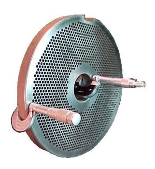
Examine the grinder plate for cracks before each sharpening. If tramp metal has been ground, examine the plate very carefully. A plate that is free of cracks will have a distinctive ring if struck with a small metal rod. Strike the edge of the plate on the 30° chamfer. Do not use a mall to ring the plate, a gentle tap is sufficient. Plates that are cracked will not ring well, and often you will simply hear a thud.
