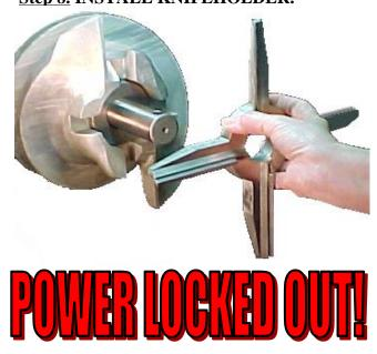
The knifeholder with fresh inserts simply slides over the pin and contacts the spring. The inserts face out! Be careful, the inserts are sharp.
