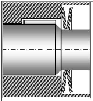
In the above illustration notice that the face at the outer diameter of the first spring is touching the counter bore in the face of the feedscrew. The second spring is opposite and will contact the knife in the same fashion. Do not stack the springs one on top of the other like dishes, this doubles the spring force and will provide too much force against the knife inserts. Do not use more than two springs.
