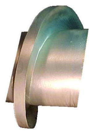
On a new or rebuilt feedscrew you will notice that the flighting is thicker. When new or rebuilt, the corners are square. Notice the nice filet welds attaching the flighting to the shaft.
