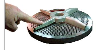
The combination of the insert slot angle and the angle that the inserts are ground provide that only the leading edge of the knife insert contacts the plate. This slight amount of clearance allows the insert to seat within a few revolutions of the grinder being turned on. The amount of material removed from the leading edge of the insert is not measurable, but it is advised that the first product that comes out of any meat grinder on start up is discarded.
