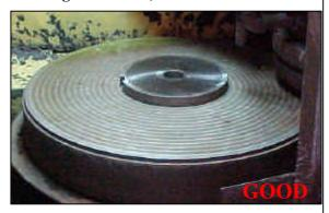
The sharpened grinder plate should have fine lines extending from the outer edge, through the center of the plate, then back to the outer edge. In drafting terms the symbol would be
