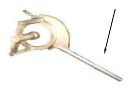
When the ring is tightened, back it off 1/8 to 1/4 turn for fine grinding, 1/2 turn for coarse grinding.
