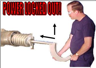
When using the ring wrench to install the feedscrew, lift the feedscrew slightly while pushing it in.
