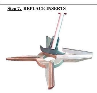
Inserting the pointed end of our insert remover into the slot of the knifeholder provides a quick and easy way to remove the knife inserts. Removing them in this manner minimizes damage to the insert locating pins found in the bottom of the insert slots in the knifeholder. We recommend starting with fresh inserts at every plate change! This includes when turning the plate around.
