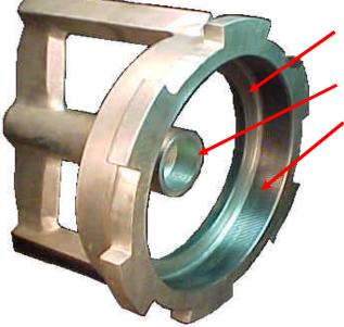
The threads are right handed, so turning the ring clockwise screws it on the head. When you can not turn it further use the ring wrench to tighten it.
