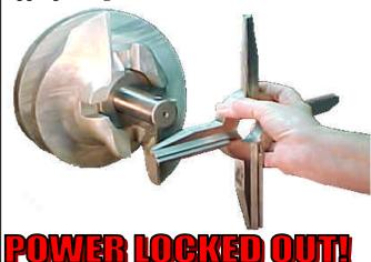
**<u>Step 5.</u> REMOVE SPRINGS:** Remove the Belleville springs, 2 each. Some pins have a spacer collar behind the Belleville springs, if this collar is used, remove it also.
