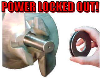
**Step 6.** INSTALL SPRINGS. The Belleville springs are installed with one spring facing down, and the second facing up toward the back surface of the knifeholder, which will be installed next. 12
