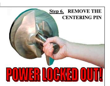
Do not loose the pin key when you are removing the pin!
