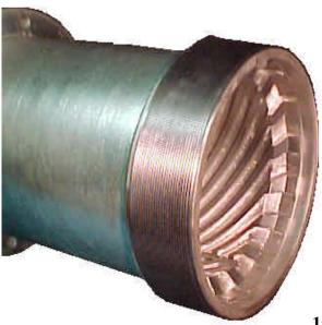
**Step 14. INSPECT THE RING** The threads of the ring should be inspected before the ring is assembled on the head. The threads must be perfectly clean, and free of any nicks or burrs. If there are nicks or burrs they must be removed or the ring and head may lock together.
