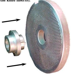
**<u>Step 12.</u>** INSTALL PLATE AND BUSHING INTO GRINDER UNIT.
