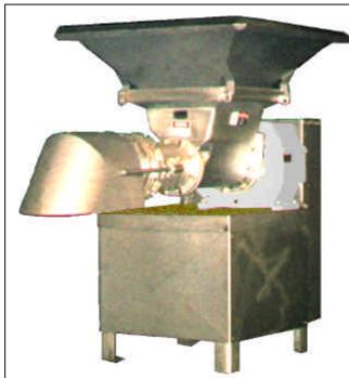
**Step 16.** INSTALL THE PLATE GUARD. Slide the rods of the plate guard into the clamps mounted to the head and tighten the wings nuts.
