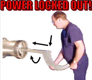
If the feedscrew does not slide up on the spline, it may be necessary to push down, in, while turning the feedscrew slightly to engage the drive spline. B drives engage much easier than the older A drives. The feedscrew will jump in another inch when it is seated on the spline. **<u>Step 5.</u>** INSTALL CENTERING PIN. Inspect the pin to make sure it is clean and free of nicks and burrs. Replace the pin when it shows wear grooves, checks, or is worn.
