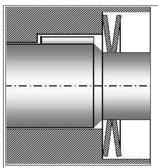
In the above illustration notice that the face at the outer diameter of the first spring is touching the counter bore in the face of the feedscrew. The second spring is opposite and will contact the knife in the same fashion. Do not stack the springs one on top of the other like dishes, this doubles the spring force and will provide too much force against the knife inserts. Do not use more than two springs.
