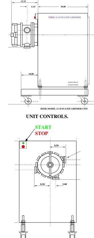
We have located the Stop-Start station on the front left side of the machine. We strongly recommend that additional stop stations are located where deemed appropriate.
