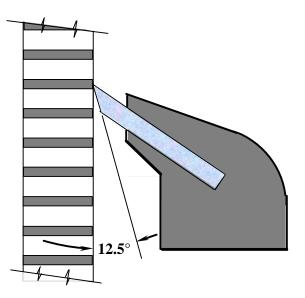
If inserts are not properly installed, excessive clearance will result.
