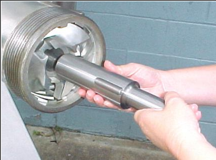
Step 7, continued. Remove the Centering Pin, don't loose the key!
