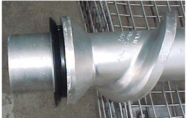
Step 9. Remove the excluder seal.
