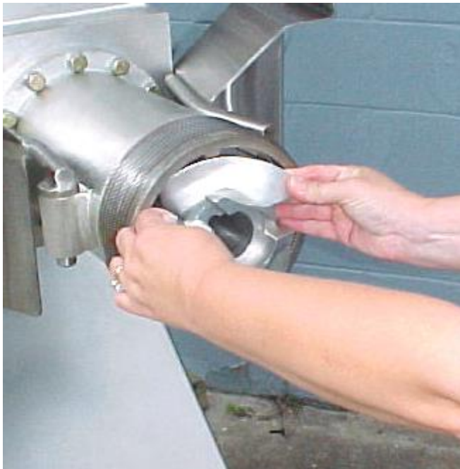
Step 8. Remove the feedscrew. Get help if it is too heavy for you.
